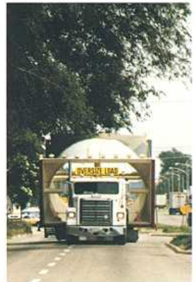
14 ft. dia. breeching on specially designed trailer
